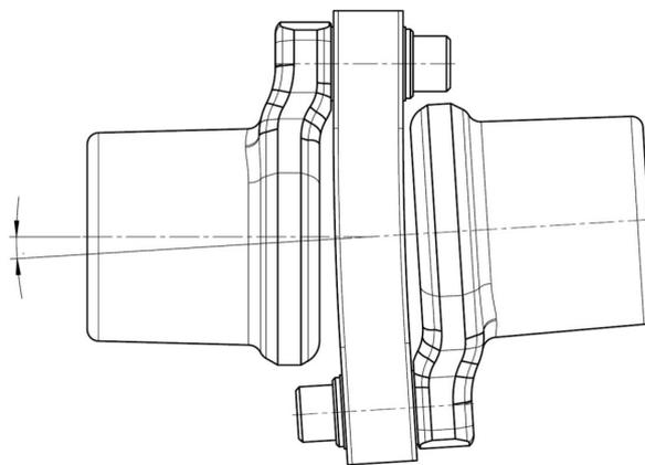
**Figure 4: Angular displacement**
