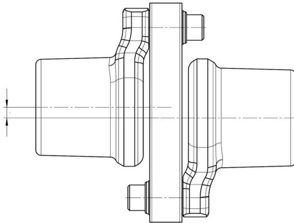
**Figure 2: Radial displacement**
